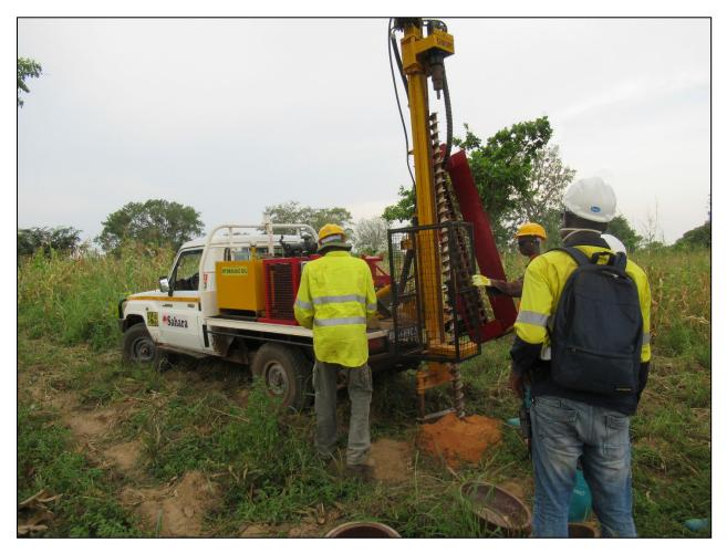
Figure 2: Auger rig drilling during phase 1 auger program
