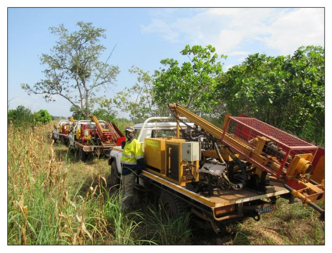
Figure 6: Three of five of auger rigs used in phase1 auger program – A fleet of five rigs is scheduled to begin drilling in late January to commence phase 2
