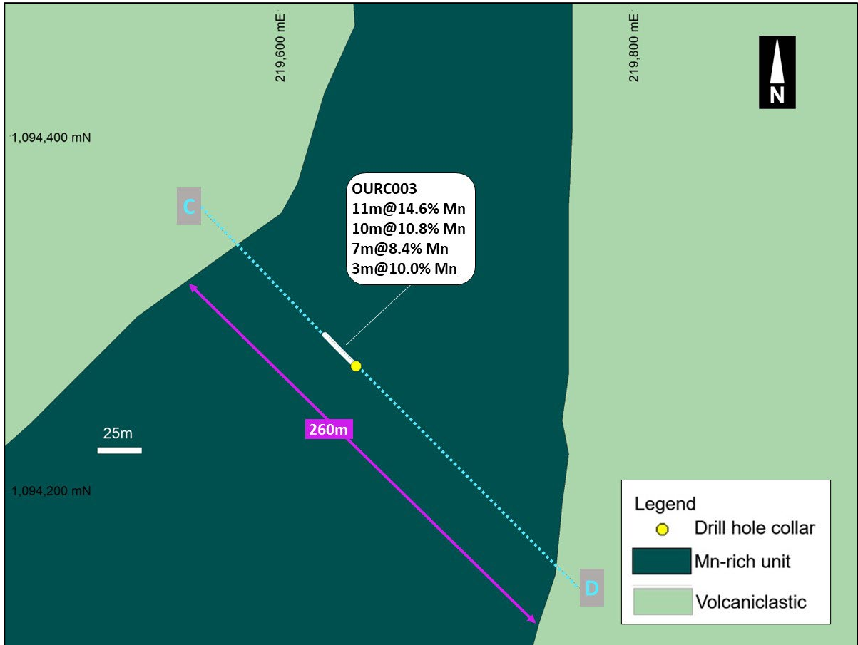
Figure 6: Drill hole OURC003 which intersected 31 metres of manganese in the 50 m hole – section line shown in blue
