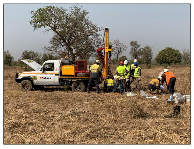
Figure 3: Type of auger rigs to be used on Napié Project which was successfully used on the Korhogo Project earlier this year
