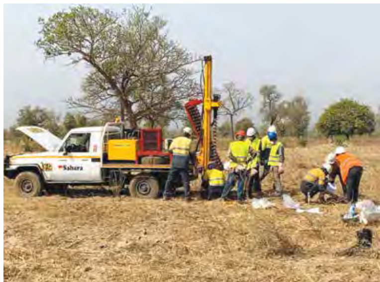
Mako is undertaking auger drilling at its Korhogo (pictured) and Napie projects in Cote d'Ivoire
